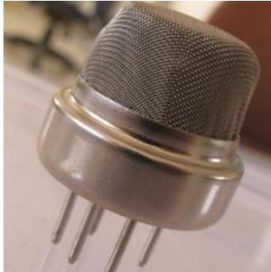
Fig. 6 Gas Leakage Sensor
